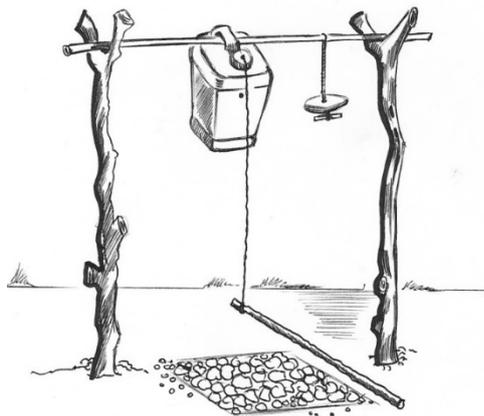
handwashing should be made as convenient as possible. Simple handwashing devices can be made from locally available materials (see illustration). Put and keep a handwashing device and cleansing agent beside the latrine, and if possible, also outside the kitchen or food eating area to provide a visual reminder to practice this behavior. Group handwashing stations in school are a good way for pupils to gain lifelong good habits through daily mandatory group handwashing.
