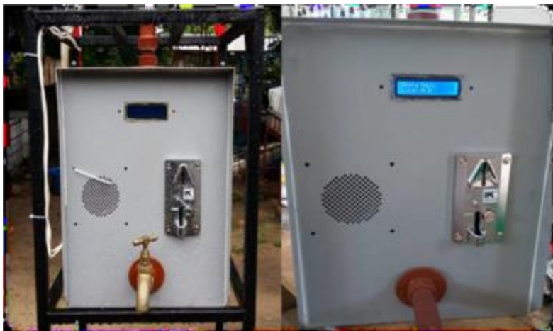
The water vending machine with built-in hygiene promotion system of UFUNDIKO
